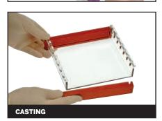
'Plug-and-Go' casting – moulded casting dams clip easily onto the ends of the gel tray for rapid external casting, allowing the multiSUB™ unit to remain in use for gel running. Casting is as simple as 1, 2, 3... place one dam onto the lab bench facing upwards and insert the tray into the groove in the dam (1) and repeat with the second dam at the other end (2). The tray is now sealed and may be placed on flat bench space or gel levelling table in readiness for leak proof gel-casting (3).
