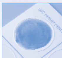
Positive Prolex® CM-MP reaction showing distinct clumping with full clearing against a white background.
